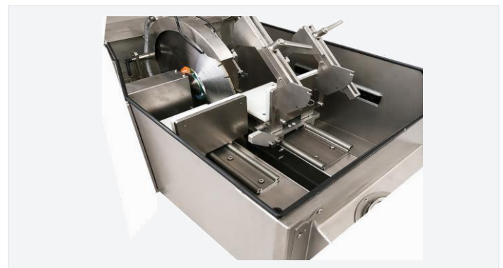
INTERNAL VIEW — DIAMOND BLADE & CARRIAGE
